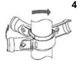
Take the first half of an MPC clamp and slide onto the ring, starting where the protruding tabs were joined in Step 1, open side of the clamp toward the open side of the ring. Slide around the rim until it locks against the pressed lug.
